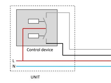
When an power outlet or other constant Live and Neutral are available near the Shuttle<sup>®</sup>, the motor can also be powered directly from the outlet. The power plug, attached to the secondary unit, can then be removed.
